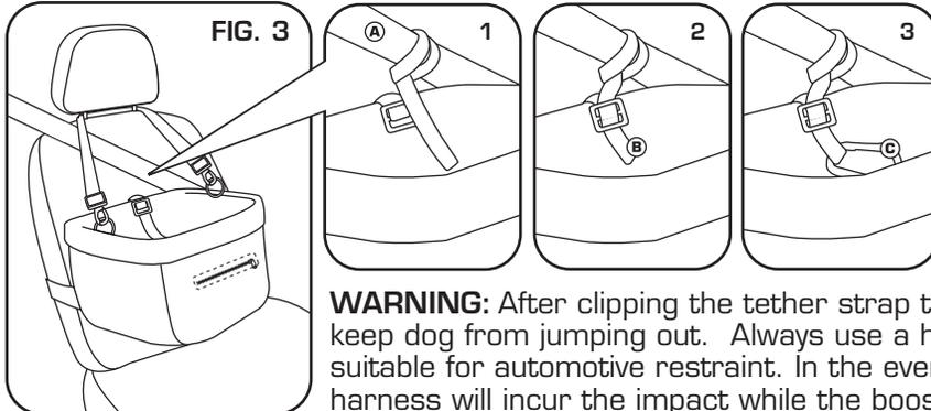
**WARNING:** After clipping the tether strap to a dog harness, adjust the length of the strap to keep dog from jumping out. Always use a harness with the booster seat, collars are not suitable for automotive restraint. In the event of an accident the seatbelt, tether and safety harness will incur the impact while the booster seat frame is meant to break away. Should an accident occur the booster seat should be replaced.
